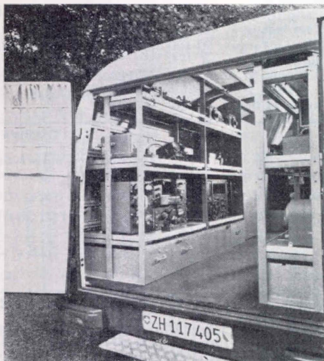
Interior of the station wagon, showing the tables securely installed for transporting.
